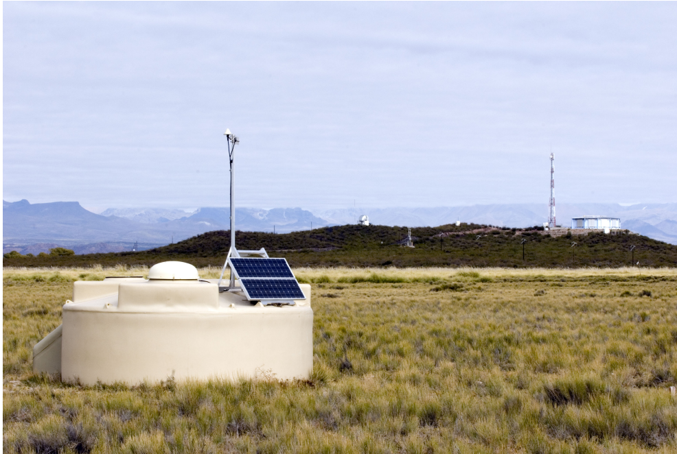
Figure 3.2: Photo of a station of the Surface Detector. A communication antenna, a GPS module, and a solar panel are clearly identifiable on top of the station. One of the sites of the Fluorescence Detector is visible on the hill far away.
