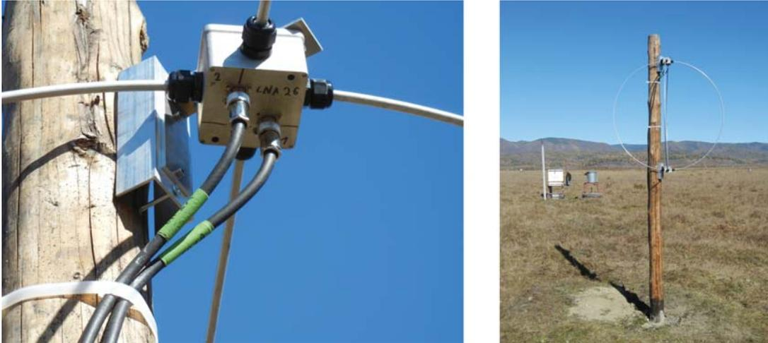
Figure 4.6.: A Tunka-Rex antenna station.
