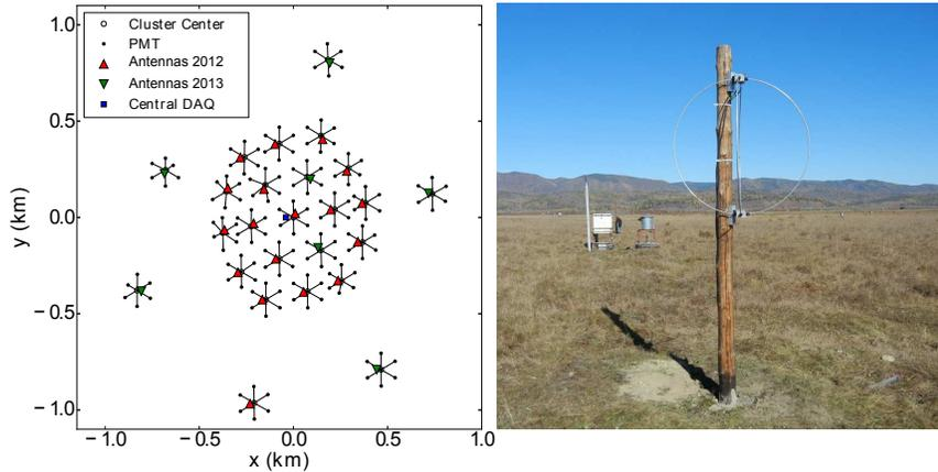
Fig. 1. **left:**Map of Tunka-133 and the Tunka-Rex antenna layout.**right:**A Tunka-Rex antenna with the Tunka-133 cluster center and central PMT in the back.
