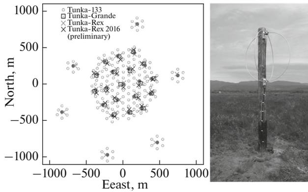
Diagram of the Tunka-133, Tunka-Grande, and Tunka-Rex facilities with provisional coordinates of the new antennas (left) and an external view of an antenna used in Tunka-Rex (right). Tunka-Rex was modernized in the period 2012–2016.
